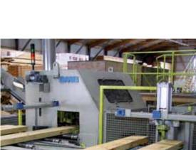
The electronic defect-cut-off saw type SKS 550 is used when smaller wood quantities are handled.
