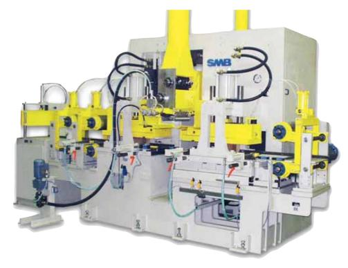
For more than 20 years the compact finger-jointing automated line type FLP is the most successful machine SMB offers for production of construction timber and laminated wood. Ranges from 6 to 50 tons of press capacity enable to choose the line in accordance with the own personal need.
