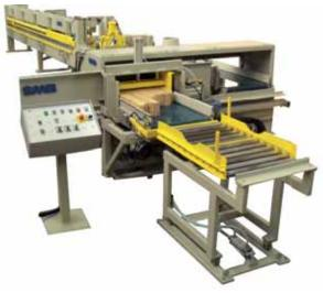
Manual rotary table erected in front of the finger-jointing machine
