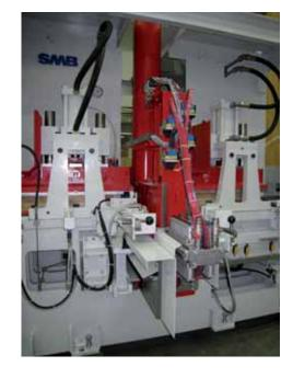
Several sizes from 20 to 30 tons of pressure capacity are at your disposal. Glue application system for all types of glue can be mounted on the machine.
