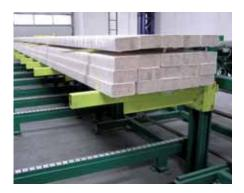
Stacking facilities with their corresponding cross storage systems for curing of gluelam timber are available in SMB normal product range.
