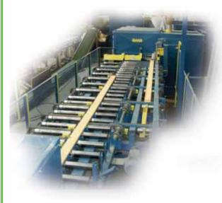
The type GFP offers a milling-press combination with contact-free glue application which finally increases considerably the output of a standard compact fingerjointing line. The line can be fitted with a glue comb. Press capacity can be chosen between 6 up to 50 tons.
